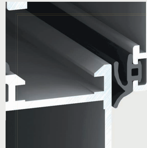
EPDM two-wing gasket that creates a tight seal between the sash and the frame when the window is closed. This prevents air and water infiltration, keeping the interior protected from external weather conditions such as rain, wind, and temperature fluctuations.
