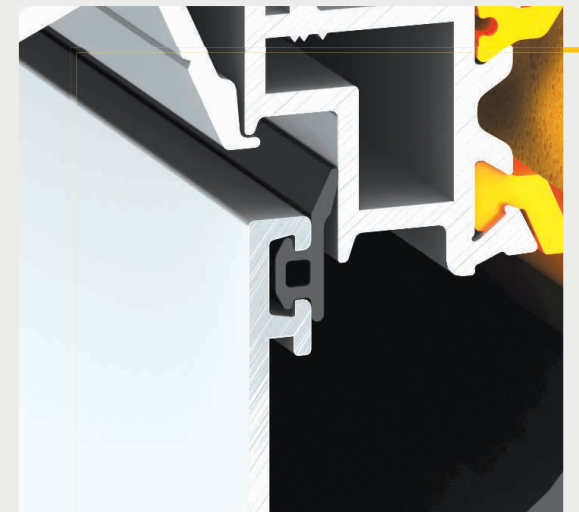
EPDM single-wing gasket that acts as an additional protective seal between the frame and the sash.
